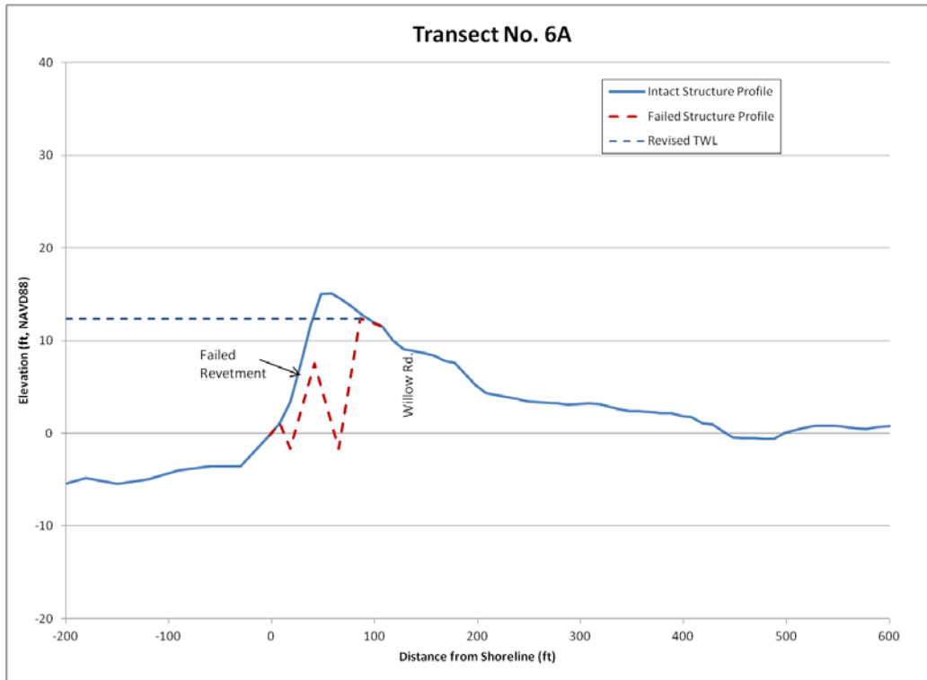
Figure 5. Intact vs. failed structure profile used to model Transect No. 6A.
